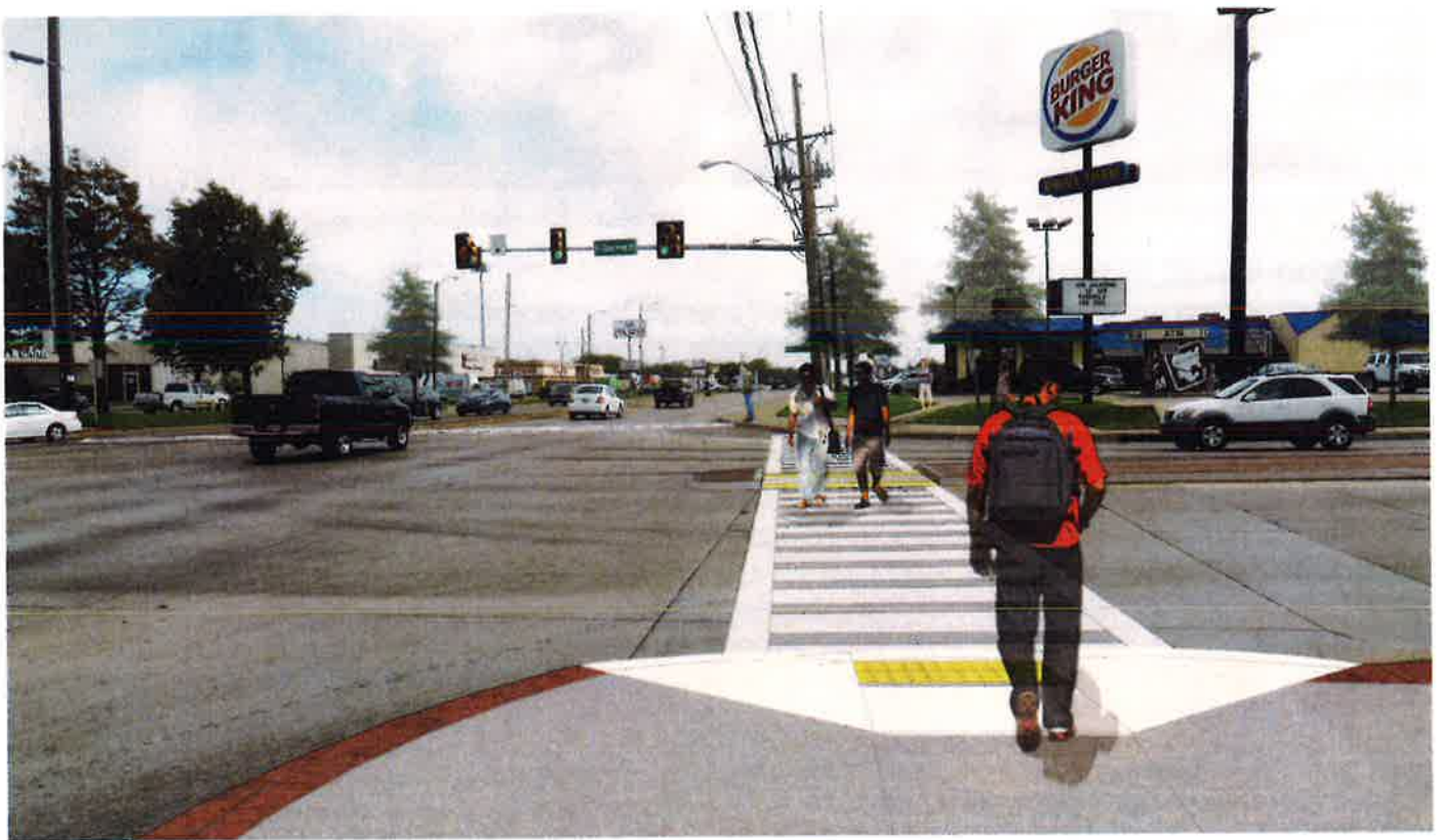
Conceptual photo-rendering of a high visibility crosswalk, re-aligned curb ramp and refuge island median
