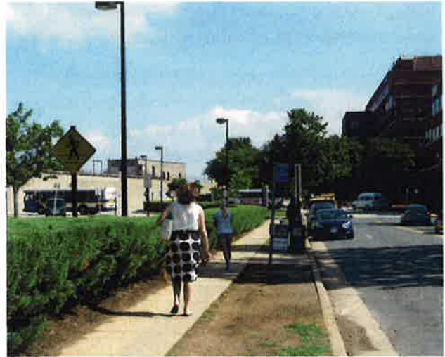
Highway-style lights (above left) serve to illuminate the automobile travel way but do not serve the sidewalk well. Parking lot lights (above right) should not be relied upon to provide sidewalk illumination.
