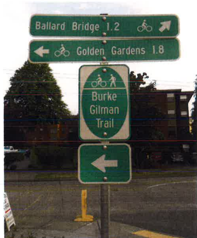
Bicycle wayfinding typically includes destination, distance and direction.
