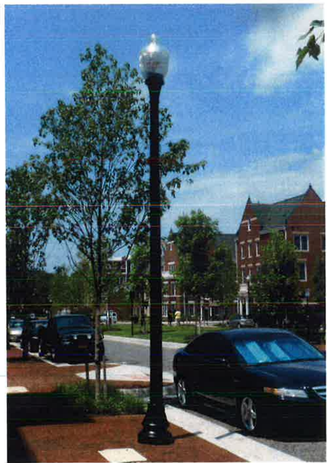
Lighting lower than 20' brings the scale of the street down to the pedestrian level.
