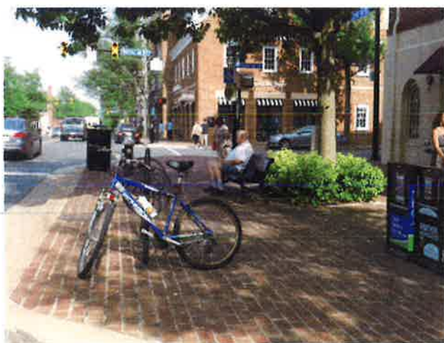
Curb extensions can be a valuable space for placing streetside amenities such as bike parking.
