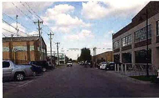
From Boulder Avenue to Main Street, a 48-foot cartpath carries two driving lanes flanked by a lane of head-in parking along the north curb. This parking should be striped as back-in @ 60° angle, and parallel parking should be added to the south curb (*Street Type 48-ADDP*).
